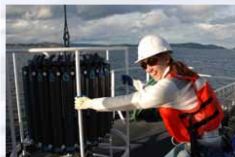
Senior Survey Technician Elaine Stuart holds onto the CTD as it comes aboard the Okeanos Explorer . Image courtesy NOAA http://www.moc.noaa.gov/visitor/photos/photospage-b/CAP%20015.jpg
