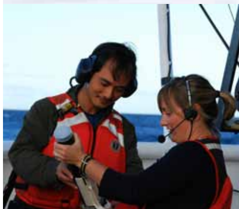
Physical Scientist Meme Lobecker teaches Indonesian scientist Cecep Sujana how to conduct an XBT cast. The XBT measures temperature through the water column. The XBT software calculates sound velocity, which is applied to the multibeam data for accurate measure of bathymetry. Image courtesy of NOAA Okeanos Explorer Program, INDEX-SATAL 2010.
