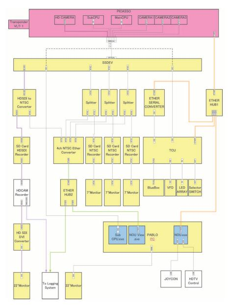
from PICASSO-1, vehicle mode (initial or dive), receipt of optical communications packets, ascent ballast drop command sent/not sent, descent ballast drop command sent/not sent, main instrumentation pressure housing leak status, power pressure housing leak status. The TCU communicates with the main control notebook computer via Ethernet and the PICASSO-1 is usually controlled and monitored within the control software (NOU, Navigation Observation Unit) and graphical user interface (NOU\_view).
