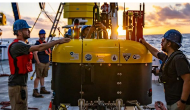
Woods Hole Oceanographic Institution's robot, Mesobot , can autonomously follow ocean animals to study their behavior. Image courtesy of Ocean Exploration Trust.
