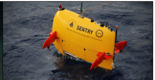
The autonomous underwater vehicle Sentry can travel to 6,000 meters depth, and carries both multibeam sonar and high-definition cameras. Image courtesy of DEEP SEARCH 2017, NOAA-OER/BOEM/USGS.
